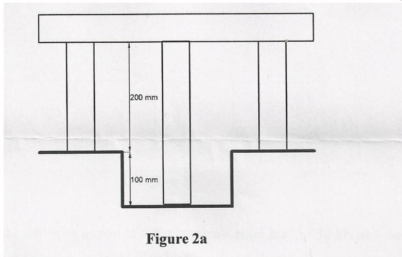
b. A compound bar made of aluminium and steel subjected to a load of 200 kN is shown in (8) figure 2. The cross-sectional area of the aluminium section is twice that of the steel section. If the elongation of the two sections is equal, determine the length of each section.
