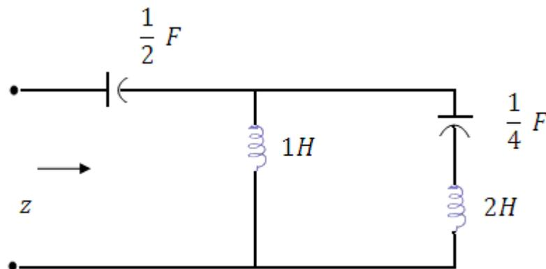
B Draw the pole-zero plot of the given network function  $V(S)$  and obtain 8
