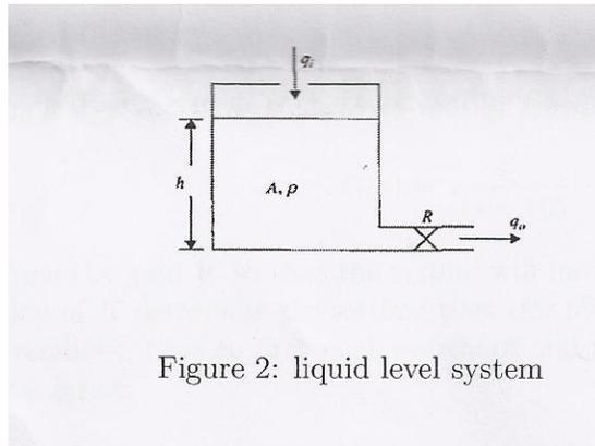
Figure 2: liquid level system
