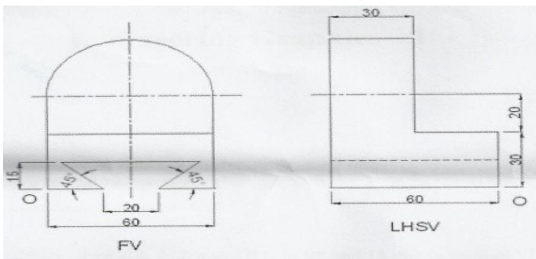
Q8 Figure 4 shows front view and end view of an object. Draw isometric view and show overall dimensions. [12]
