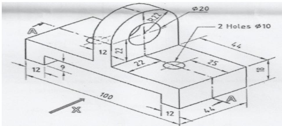
Q7 Figure 3 shows front view and end view of a bracket. Draw isometric view and show overall dimensions. [12]
