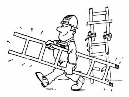
Any damaged ladder should be destroyed and replaced by a new one.
