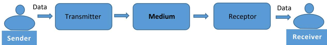
Sender who wants to send the data to receiver feeds the data to transmitter. Transmitter processes or encodes the data to generate signals which can propagate and carry the data over the medium. These signals are captured by the receptor at receiver end. Receptor decodes intercepted signals to generate original data and gives it to the receiver.
